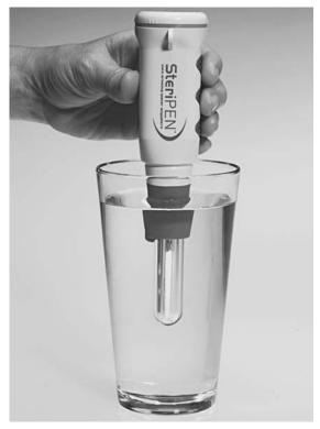
The SteriPEN is a water purifier that disinfects with ultraviolet (UV) light to destroy waterborne microbes. Operating on four alkaline AA batteries, it purifies 16 ounces of water in a minute and a half. It should be used only on clear water; sediment hinders its effectiveness. (SteriPEN)
