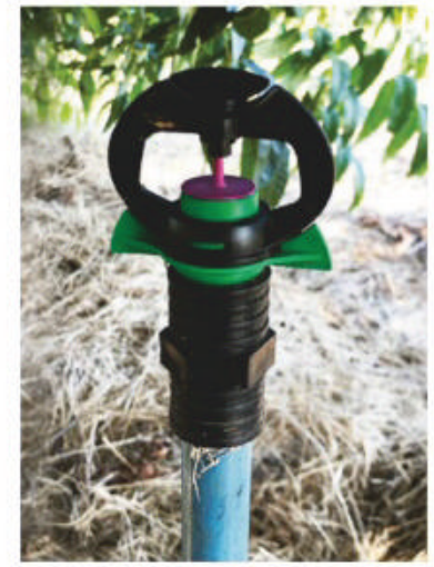
► Micro sprinkler with insect guard.
