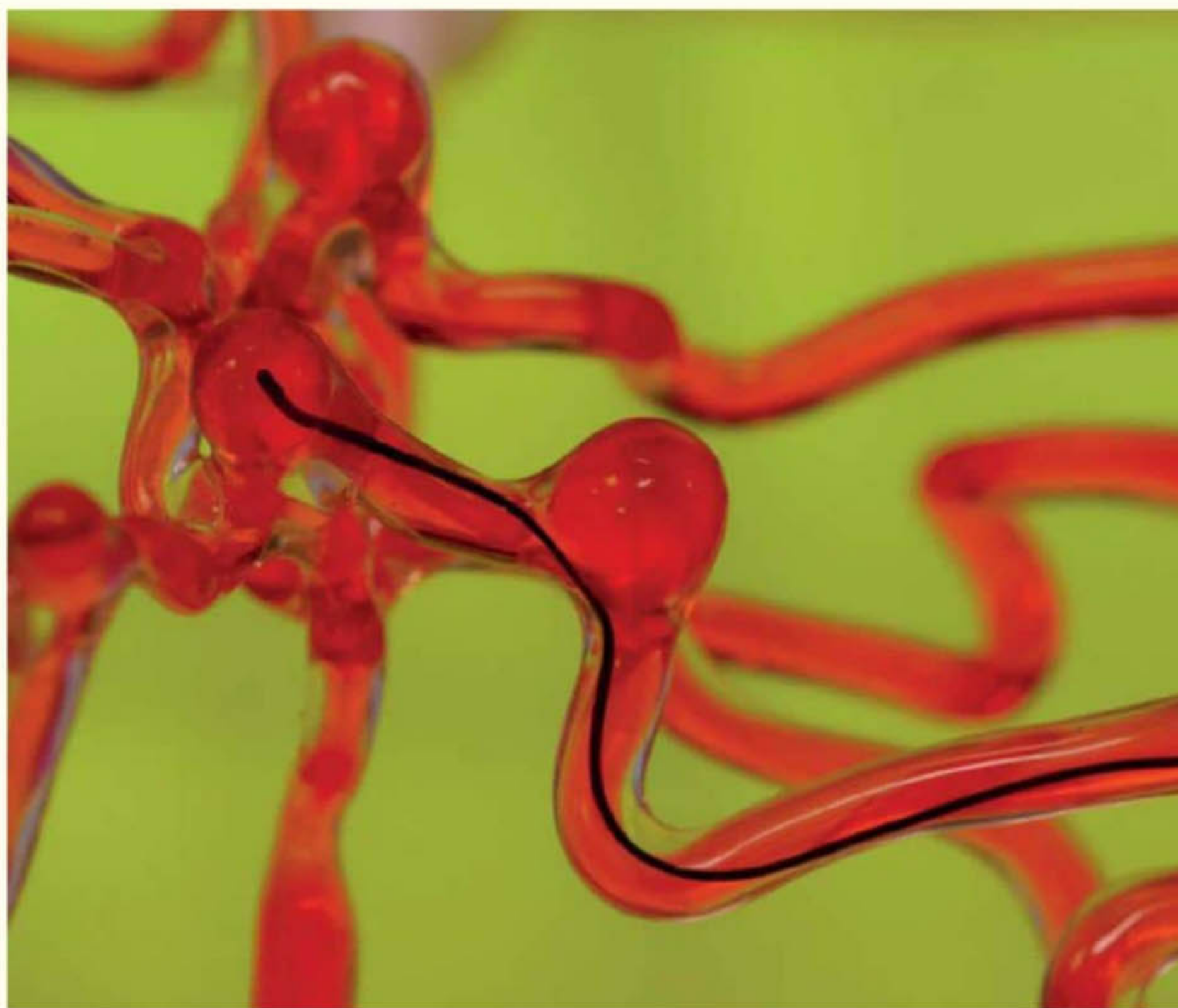
The robot was guided through replicas of blood vessels without causing damage
