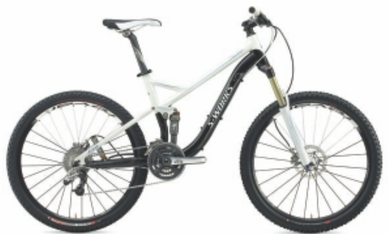
Narrower handlebars, shorter top tubes, shorter stems, and shorter cranks all give women a much more comfortable ride. (Pictured is the Specialized S-Works Safire.)
