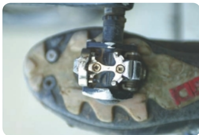
Clip-in pedals require shoes with holes in their soles to accommodate the metal cleats. When your sole wears out, the cleats make a cool “click, clack” sound on hard floors. This pedal is made by Shimano.
