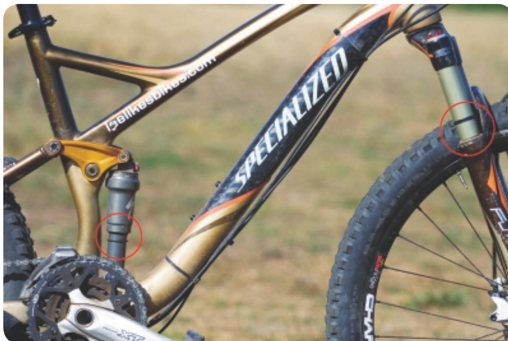
The placement of the o-ring (shock) and zip tie (fork) show the proper amount of sag for this 2008 Specialized Stumpjumper Pro Carbon.
